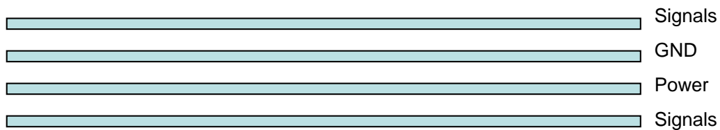
Figure 15: Typical 4-layer PCB construction
